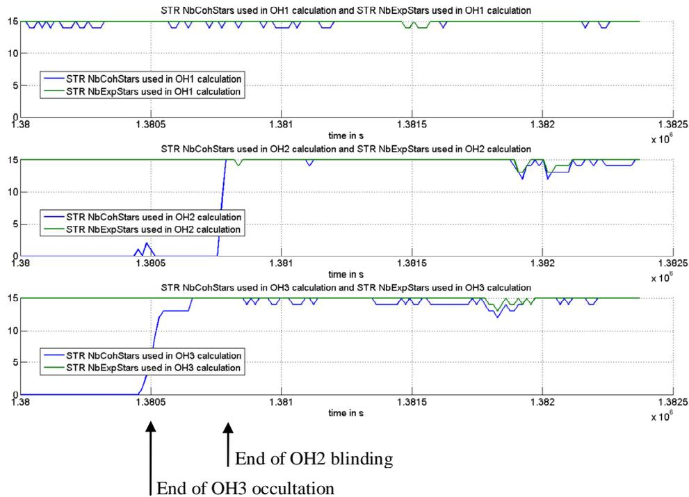
Figure 6: Number of coherent stars during OH2 Sun blinding and OH3 Earth occultation
