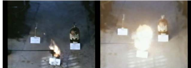
Summerfield pours aniline on to RFNA. Rapid and vigorous ignition!! Hypergolic!!
