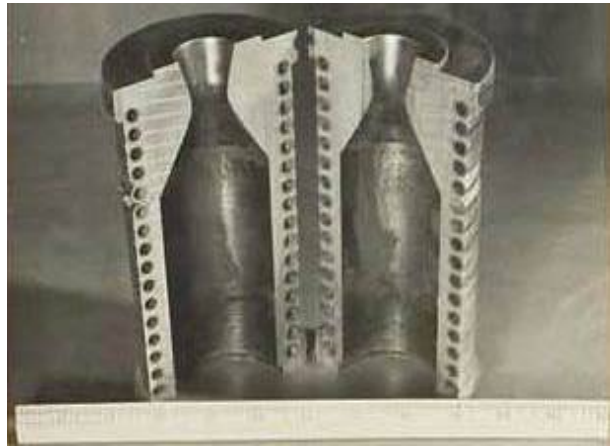
Fig. 8 Regeneratively cool chamber prototype put into practice James H. Wyld’s invention. (24 December 1941 JPL 383-177 low res)
