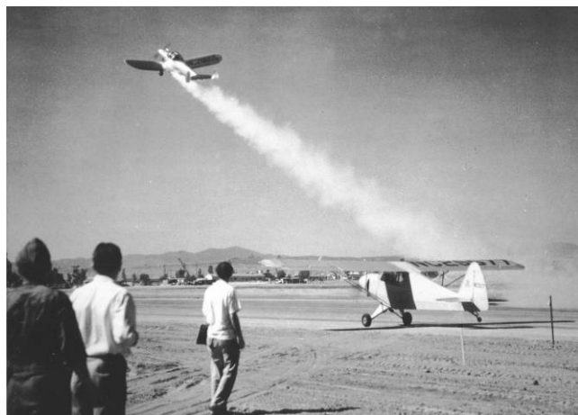
a) Ercoupe takes off with six black-powder solid propellant JATO units, each delivering \sim 0.12 kN for \sim 12 sec. First US JATO flight was 12 August 1941. Pilot Capt. Homer A. Boushey (von Kármán master's degree graduate) agreed to the risky test; a week earlier a JATO motor experienced an "explosive failure" in level flight 5
