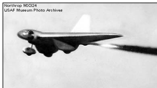
Fig. 13 Northrop MX-324 (9.8-m wing span), experimental flying wing, sustained flight with Aerojet XCAL-200 pressure-feed liquid-propellant engine on 5 July 1944, an AAF funded US first, almost three years after the successful flight of the Messerschmitt Me-163.
