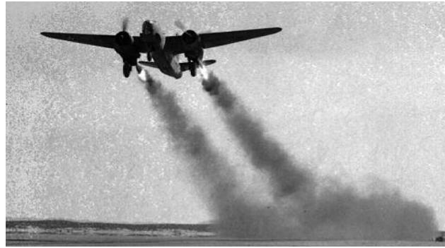
a) Douglas A-20A Havoc take-off with liquid-propellant rocket JATO from Muroc Army Air Forces Base (now Edwards AFB). (JPL 383-93 1942)
