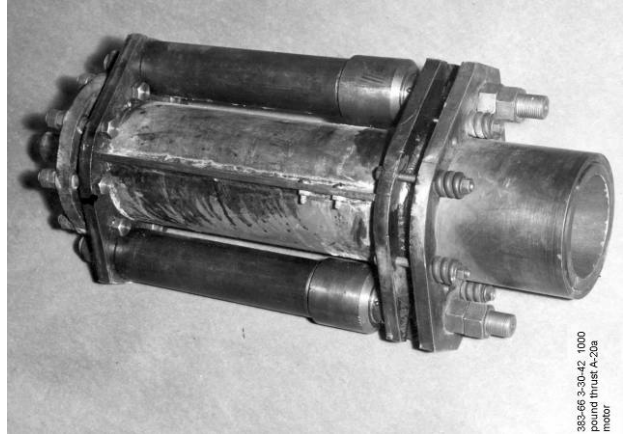
Fig. 7 The 4.45-kN engine used on Douglas A-20A had a 10.2-cm internal diameter. The schedule did allow time to qualify reduced mass hardware. (1942 JPL 383-66)
