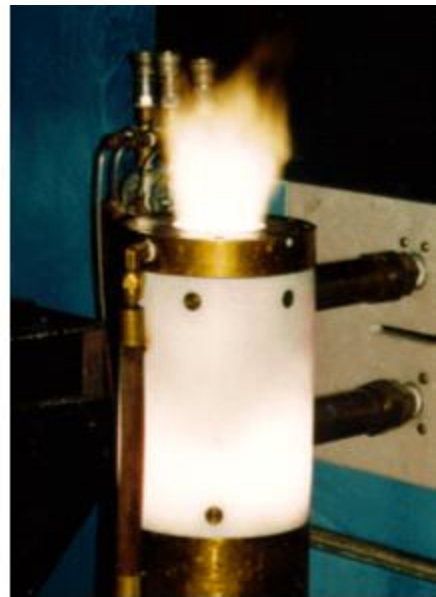
Figure 2: Torch head schematic and photograph of the air plasma plume. All measurements were performed 16 mm downstream of the torch exit nozzle [5]
