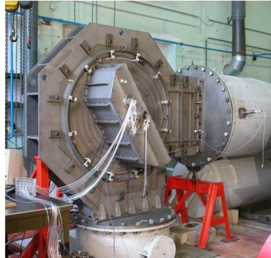
Fig. 2b – Assembly of the cascade model
