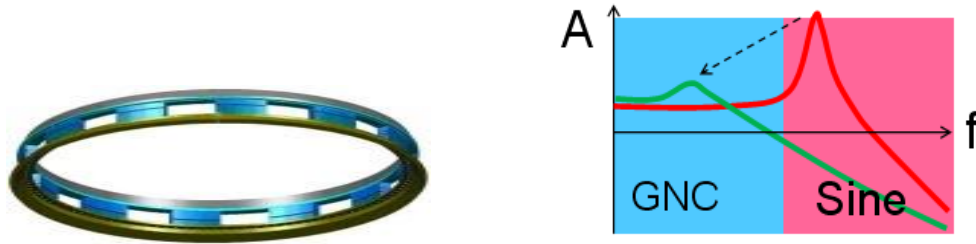
Figure 11: Passive Isolation Device (PID) principle
