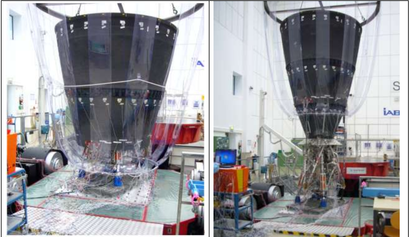
Figure 6 : Vinci engine M5 during dynamic testing
