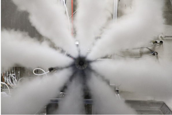
Figure 11: Test with HTP catalyst chamber carried out in December 2012 (mass flow 109,6 g/s)
