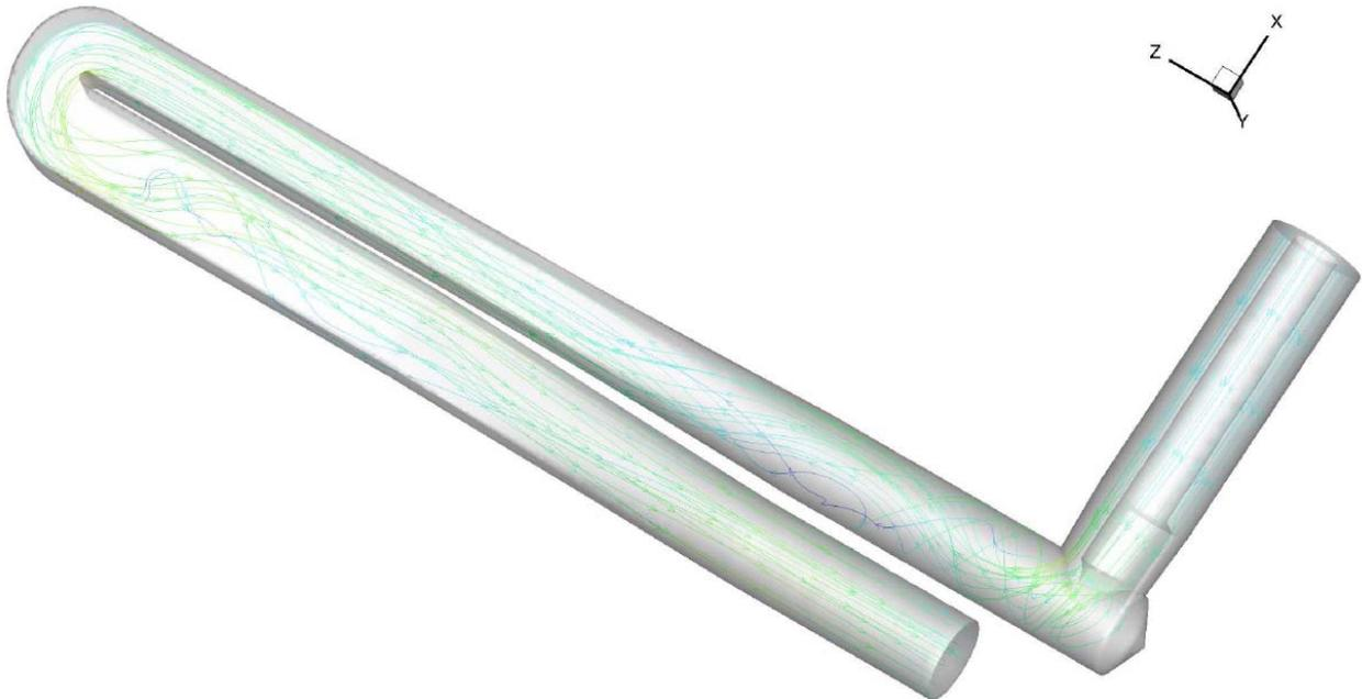
Figure 18: Streamtraces calculated in rotating configuration ( $Re=25\ 000$ ,  $Ro=0.33$ )
