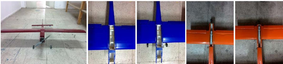
Figure 2: Photos of ZANKA-I and Its Passive Morphing Equipment
