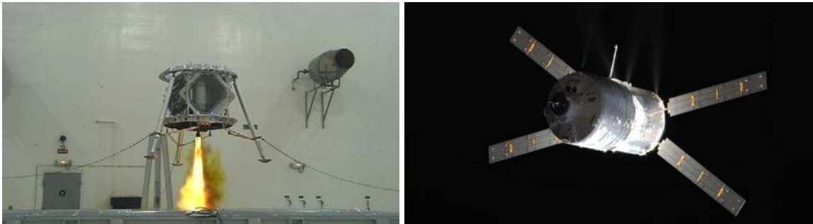
Fig. 2: HOMER MPS and ATV ACS propulsion firings
