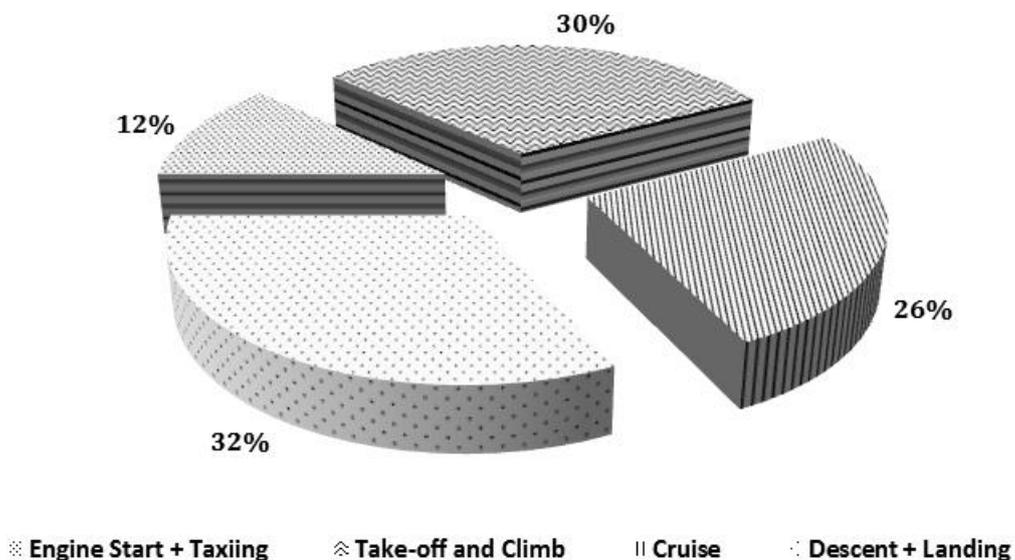
Figure 3: percentage of maximum electrical load during normal operation flight for basic electrical equipment
