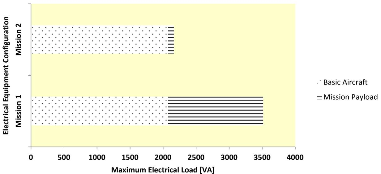
Figure 5: maximum electrical load for mission 1 and mission 2 electrical payloads
