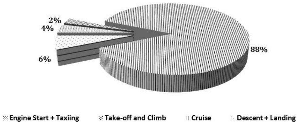
Figure 1: percentage of electrical current utilization during normal operation flight for basic electrical equipment
