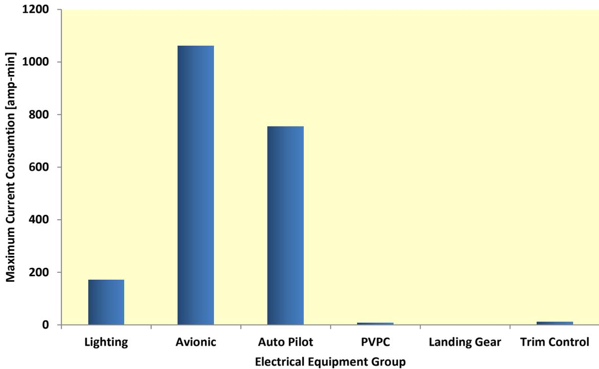
Figure 2: total maximum current for each basic electrical equipment group during cruise
