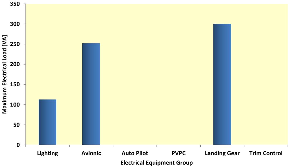
Figure 4: total maximum electrical load for each basic electrical equipment group during descent + landing
