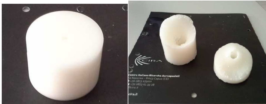
Figure 13: Picture of the paraffin grain manufactured with the heated and pressurized metallic box.
