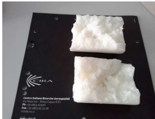
Figure 12: Internal surfaces after sectioning of paraffin wax solid grains manufactured without application of external pressure.
