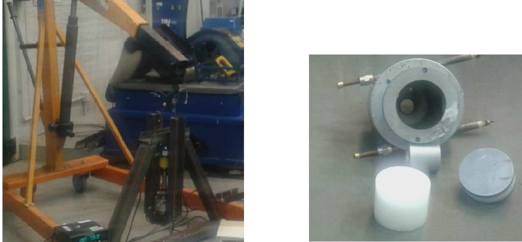
Figure 12: Metallic box, heated through electrical resistance and pressurized with oleo-dynamic piston used to manufacture the paraffin grain.
