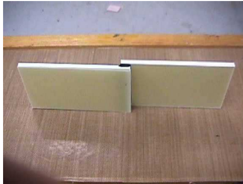
Figure 9. Lap shear specimen bonded with structural adhesives
