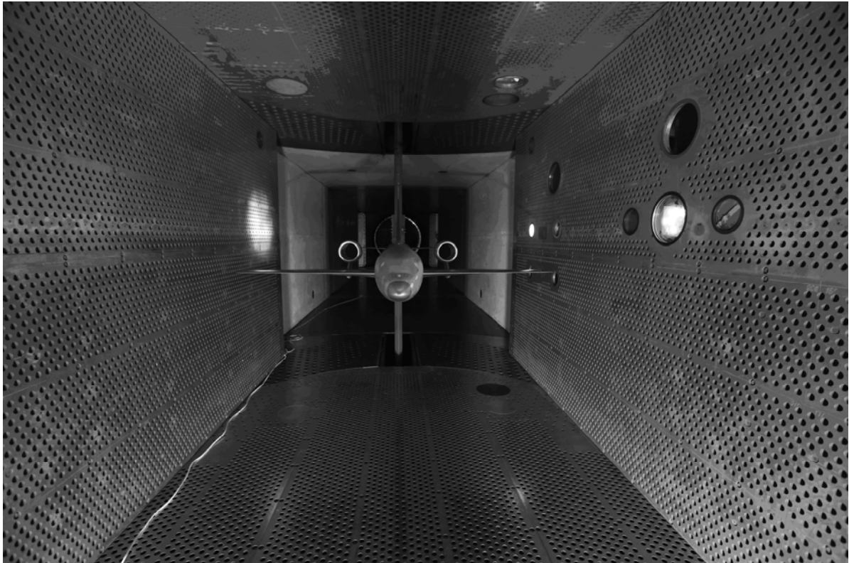
Figure 7: Model of low-noise configuration in transonic wind tunnel
