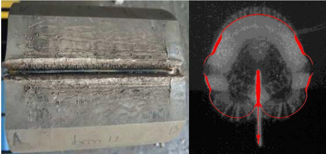
Figure 9. Penetration of RDX/Copper Linear cutting cords (left) and superposition of flash X-Ray and numerical simulation of cutting cord expansion (right) [19]
