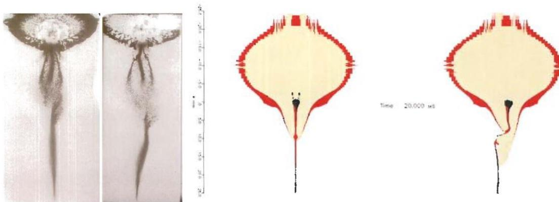
Figure 8. Comparison between X-ray imaging and numerical simulation for suspicious detonating cords [18]
