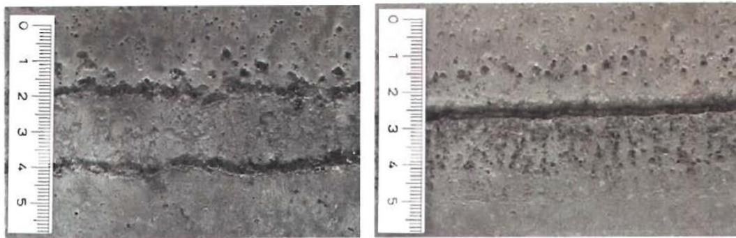
Figure 7. Penetration target on aluminium plate with suspicious and standard lead cutting cord [18]
