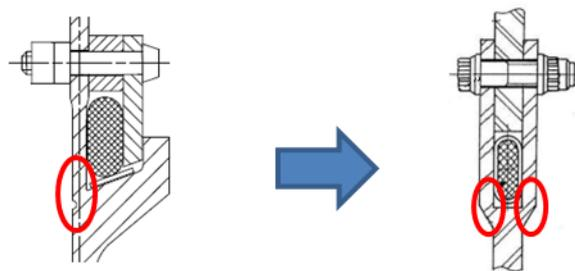
Figure 6. Configuration change for fairing separation system [4][5]
