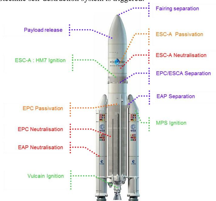
**Figure 1. Pyrotechnic functions**
