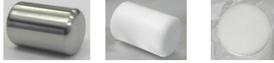
Figure 3: Left: cylindrical stainless steel sample; middle: cylindrical PTFE sample; right: disc-shape PTFE sample
