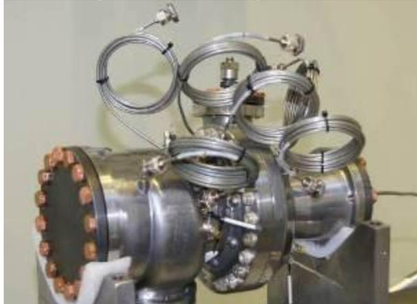
Figure 12. AVIO Fuel TurboPump Assembly
