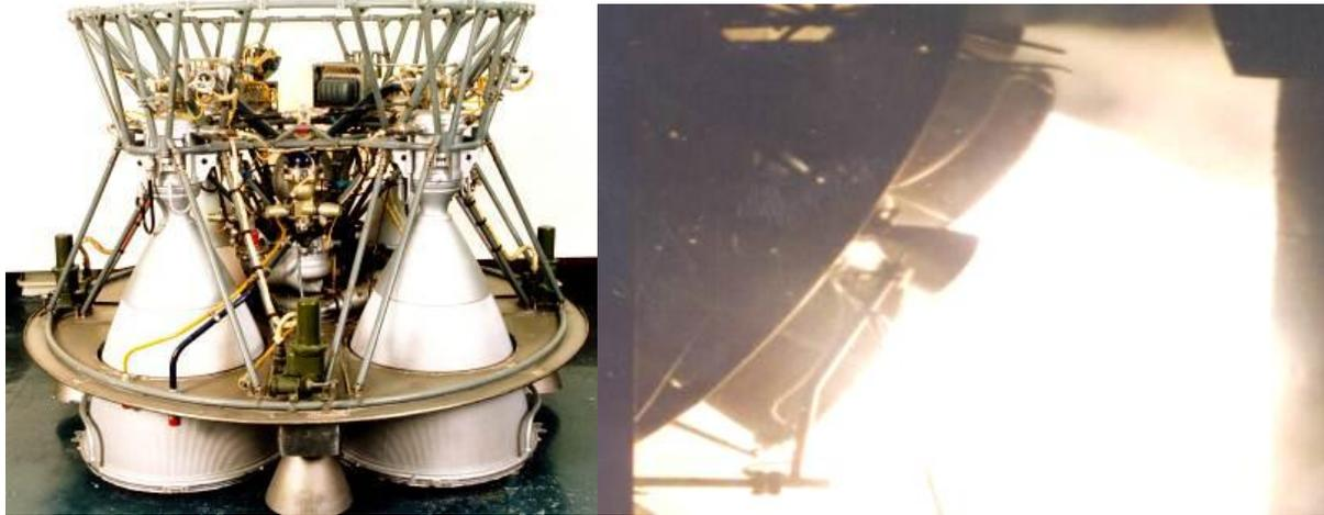
Figure 1. RD0110M engine and its fire test at KBKhA's test facility
