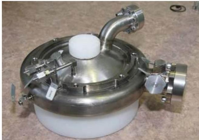
Figure 8. LM10-MIRA Injector Head
