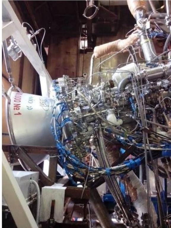
Figure 17. LM10-MIRA Demonstrator on the test stand
