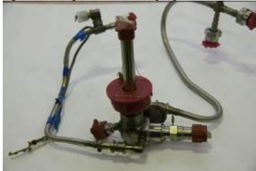
Figure 14. – The igniter device
