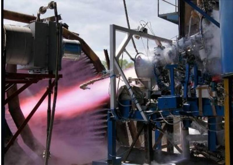
Figure 20. LM10-MIRA Demonstrator engine fire test
