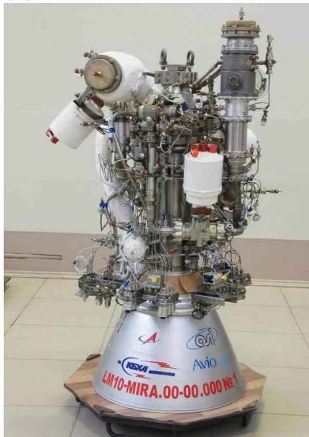
Figure 16. LM10-MIRA Demonstrator Assembly
