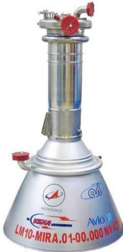
Figure 9. External view of the Thrust Chamber Assembly
