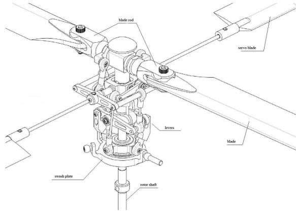
Fig. 1. The main rotor hub of the Hiller type
