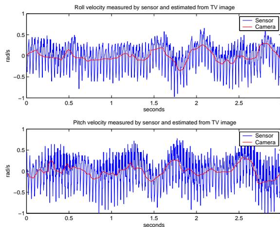
Figure 3: Angular velocities measured by the onboard sensor and by TV cameras
