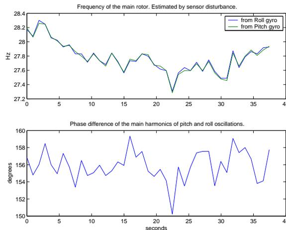
Figure 5: Estimates of frequency and phase of the main rotor by two gyroscopes
