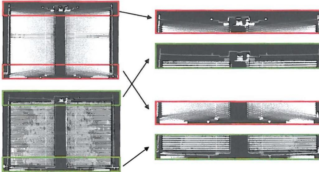
Figure 8: Section view of a CD stack via Standard CT (top picture) and Helix-CT (bottom picture). [9]
