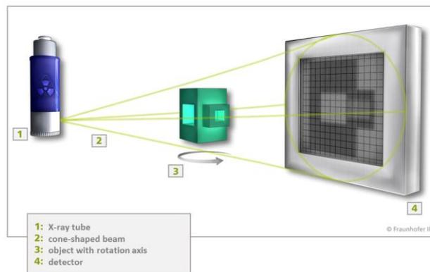
Figure 6: Standard industrial Computer Tomography based on cone shaped x-ray beam [8]
