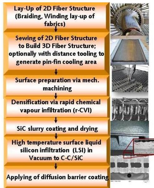
Figure 5: Schematic flowchart of the CARBOTEX<sup>SI®</sup> (C/C-SiC) via r-CVI & LSI
