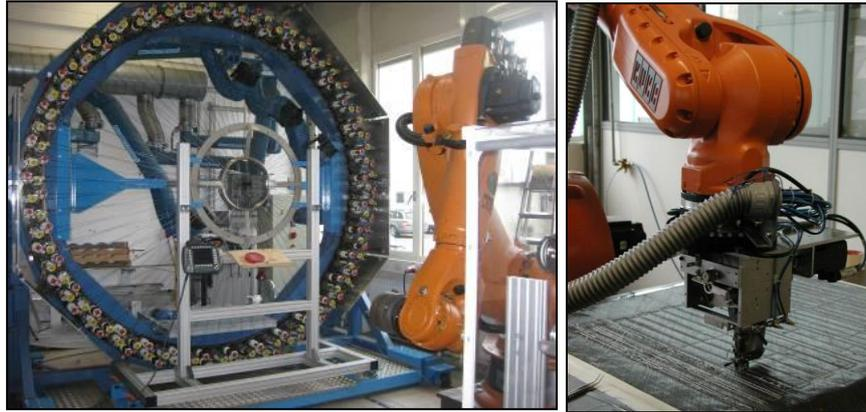
Figure 4: Robot-assisted circular braiding device (left)
