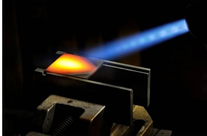
Figure 12: Hot testing of a flat material sample in ERBURIG<sup>K</sup> facility.
