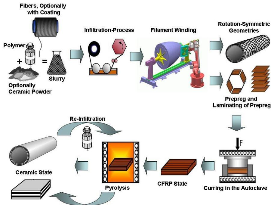
Figure 3: Schematic flowchart of the Polymer Infiltration Pyrolysis (PIP) process
