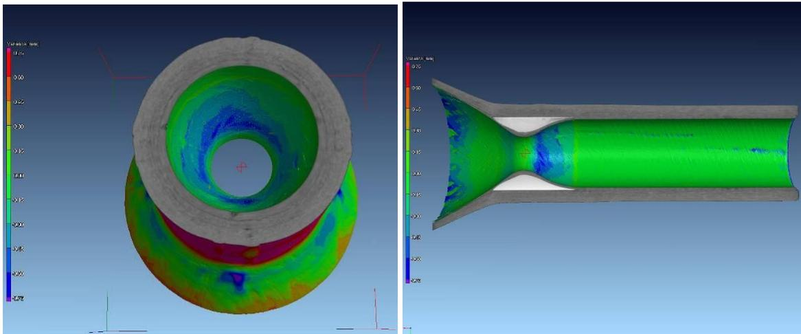
Figure 11: 3D measurement of contours and comparison with CAD data.
