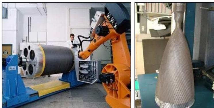
Figure 2: Filament winding facility for geometries  $> \varnothing 1.5 \text{ m} / 3 \text{ m}$  length (left)
