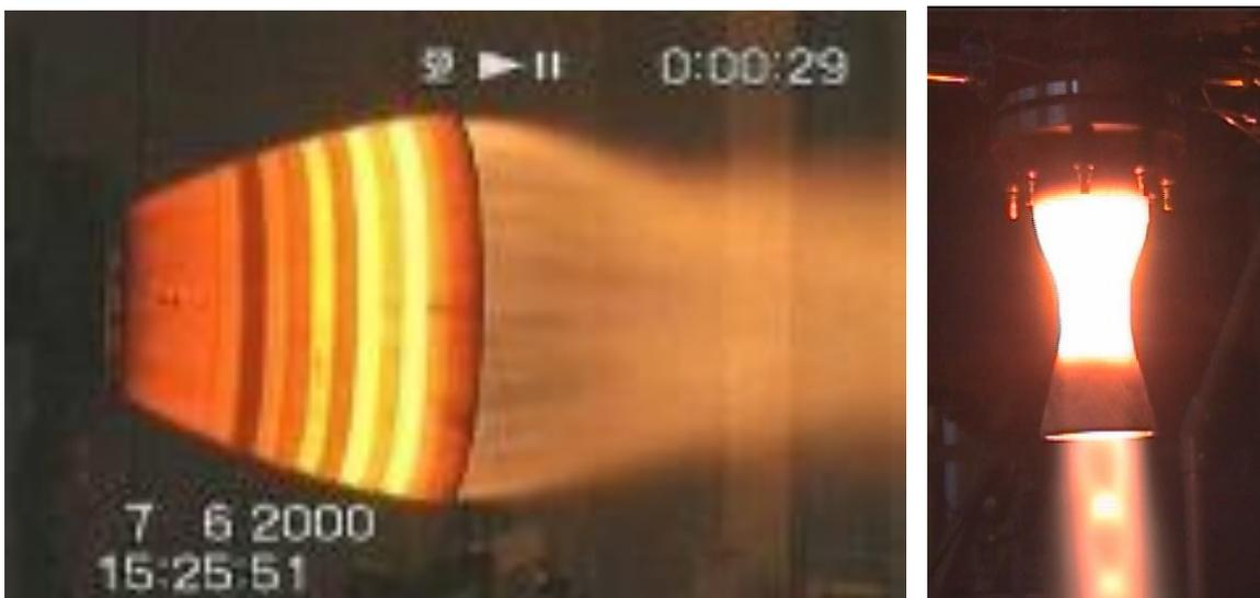
Figure 13: Hot testing of a Vulcain subscale nozzle made of C/SiC (left)
