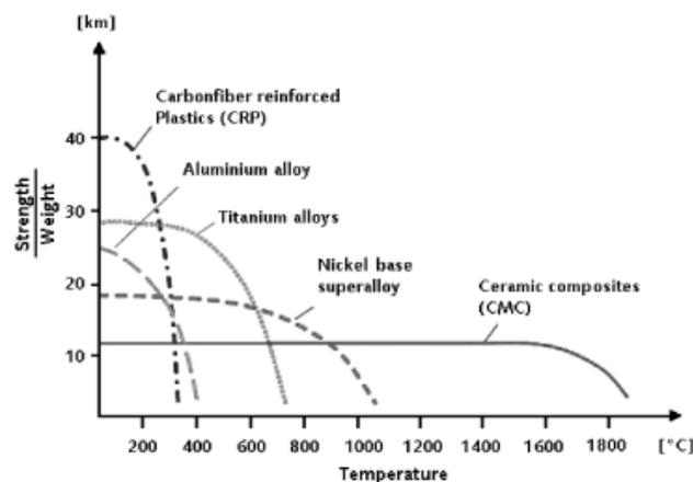
Figure 1: Ratio of strength to weight as a function of temperature [1]
