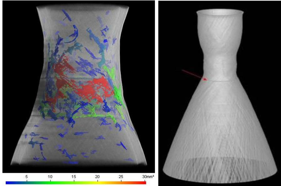
Figure 10: Detection of defects in complex shaped components.
