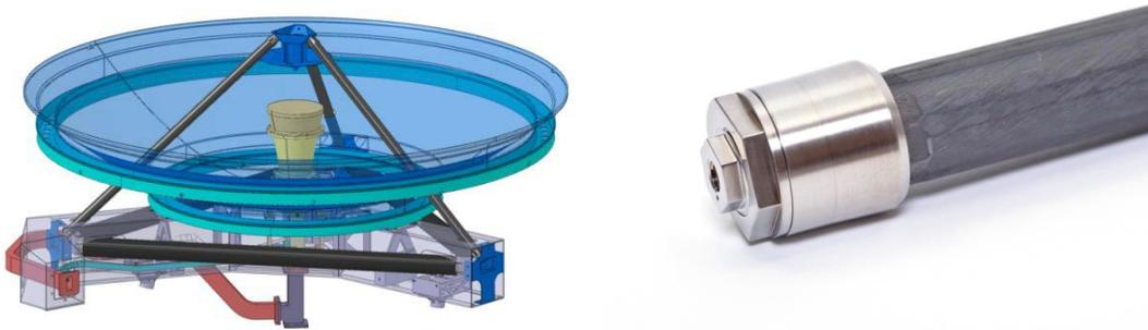
Figure 14: High Gain Antenna arrangement (left). Clamped fitting on C/SiC strut (right).
