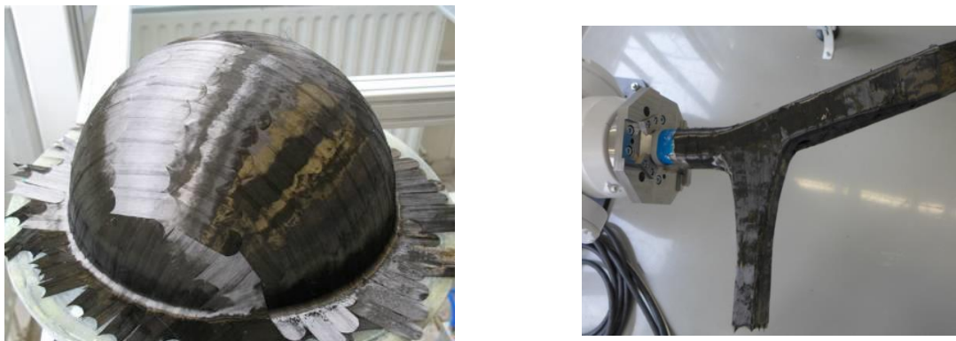
Figure 12: Illustration of complex parts manufactured with the FPP process.
