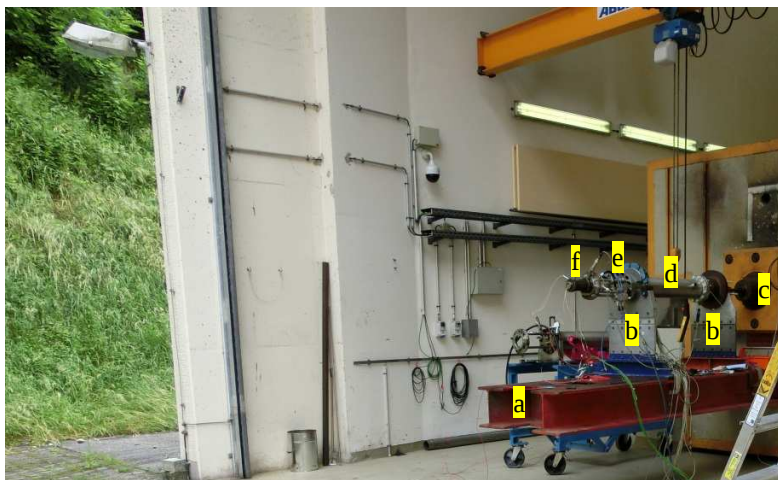
Figure 2: GRM static test facility with small GRM for propellant tests. a) main support, b) flexible support, c) thrust measurement cell, d) GRP tank 10 litres, e) GRP FMFR control devices, f) CC with injector and nozzle.
