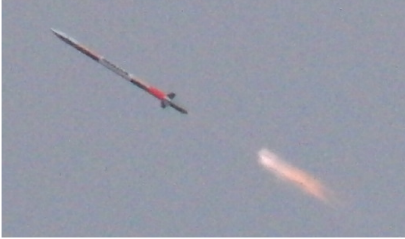
Figure 7: GRM demonstrator missile just after launch. Propellant: GRP 001, GRM with 5.5 kN nominal thrust [7]
