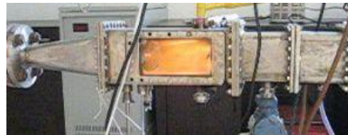
Fig.4. Stable combustion of plasma jet ignition in the combustion chamber
