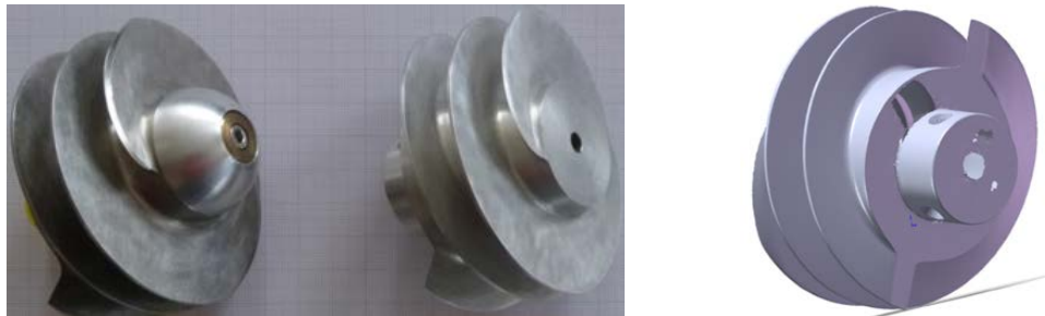
Figure 2: H2O LOX inducer: original test hardware (respectively Inconel and Aluminum) (left) and 3D-scan (right)
