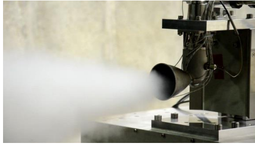
Figure 5: firing tests at DLR Tauern test center
