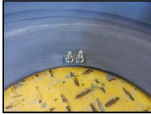
Figure 15: Potentiometers pins position and detail of the initial cracks on the small scale PTF
