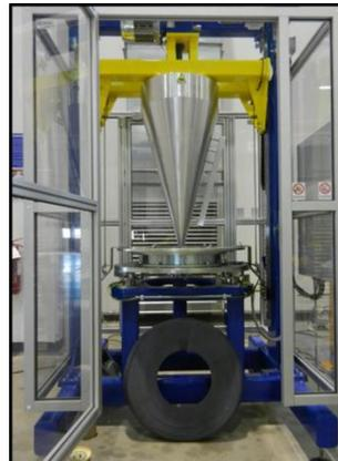
Figure 13: Testing machine used for both Mode #1 and #3 small scale tests. In the low, the small scale PTF
