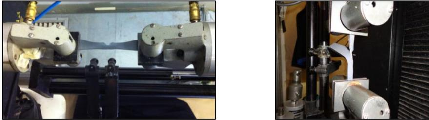
Figure 11: Mode #1 (on the left) and #3 (on the right) Tearing Tests
