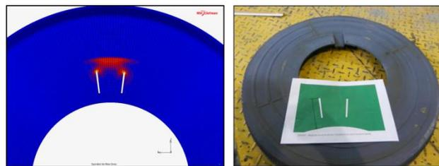
Figure 25: Crack shape and final crack length for Mode#3 break: numerical vs experimental results
