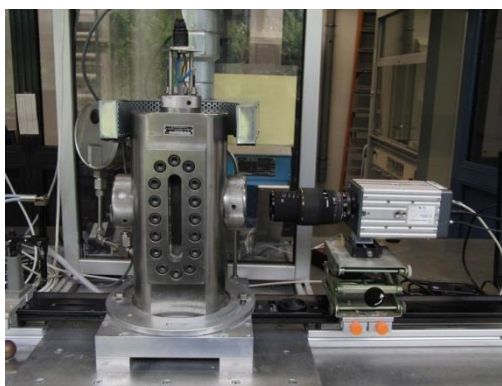
Figure 6. Experimental setup of window bomb and camera
