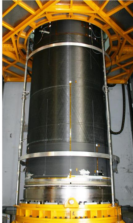
Figure 12: Z40 DM00 motor case on test bench
