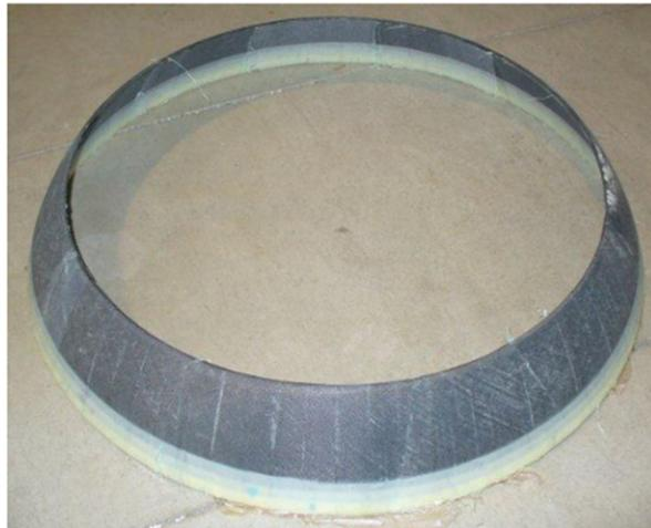
Figure 16: Prototype of hybrid composite spherical reinforcement shims at Z23 scale
