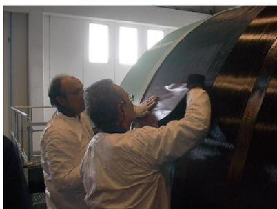
Figure 10: Manual deposition of tape
