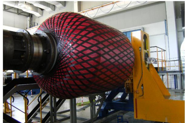
Figure 8: Avio prepreg winding on Z9 scale
