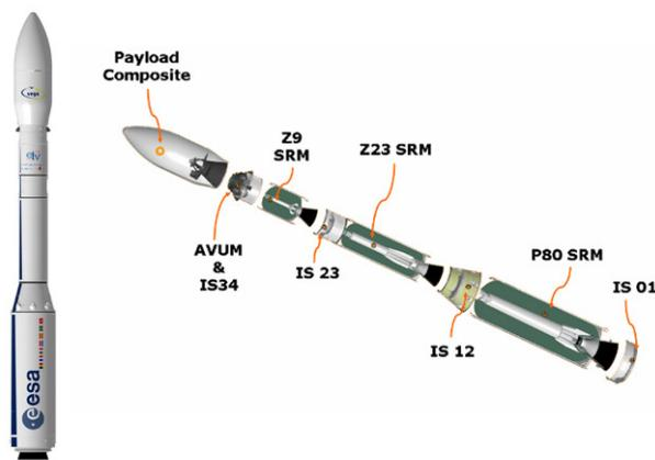
Figure 1: VEGA launcher configuration
