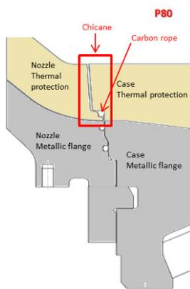
Figure 19: P80 chicane with carbon rope
