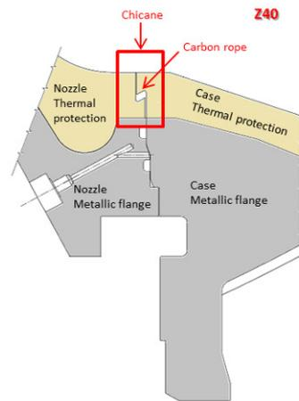
Figure 20: Z40 chicane with carbon rope
