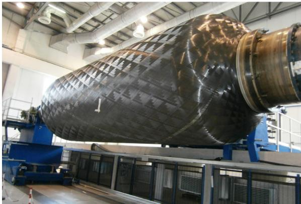
Figure 7: Avio prepreg winding on P80 scale
