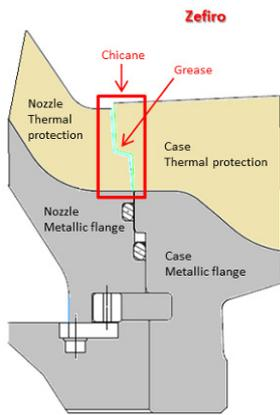
Figure 18: Zefiro chicane with grease
