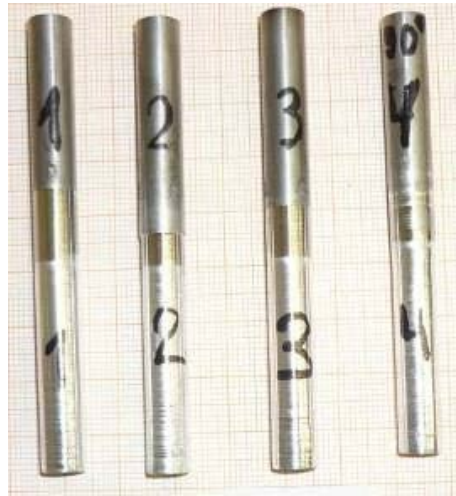
Figure 3: Examples of welded coupons prepared for tensile testing.
