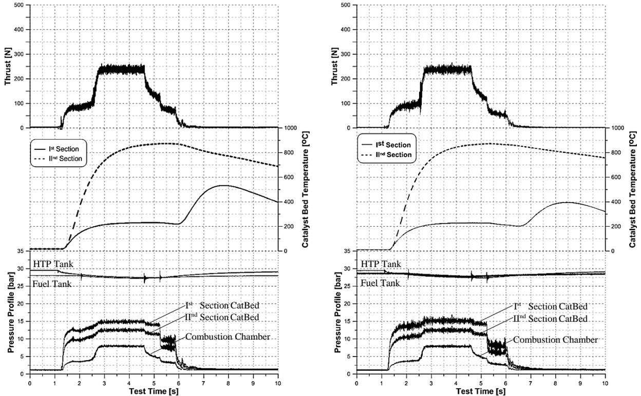
Figure 8. Measured parameters during the test of the kerosene ignition (8 injectors configuration).
