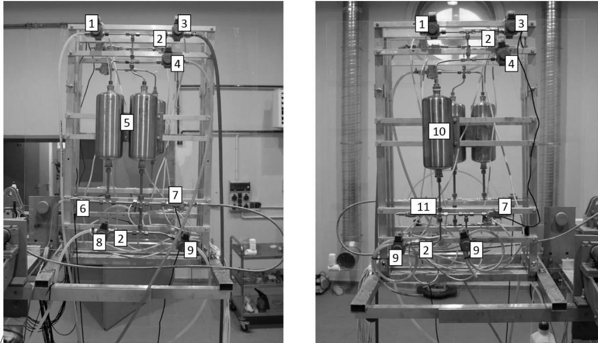
Figure 5. Propellant supply system: HTP (left) and fuel (right). 1-vacuum line valve, 2-check valve, 3-pressurizant valve, 4-relief valve, 5-HTP tanks, 6-pressure and temperature measurement port, 7-flowmeter, 8-inlet valve, 9-dump valve, 10-fuel tank, 11-pressure measurement port.
