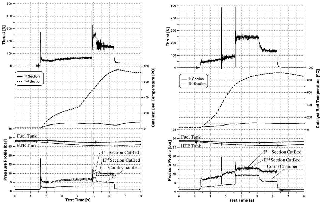
Figure 11. Measured parameters during the test of the isopropyl alcohol ignition (4 injectors configuration).
