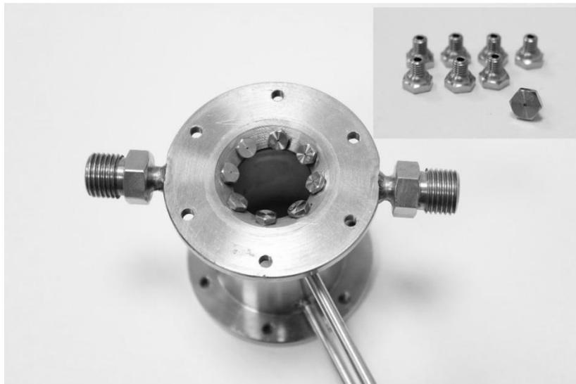
Figure 2. Catalyst chamber with interchangeable fuel injectors
