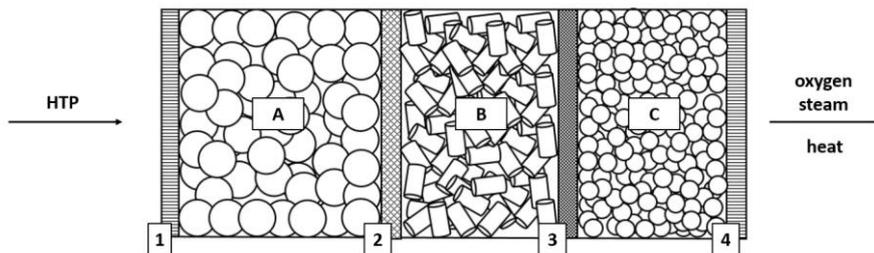
Figure 6. Composite catalyst arrangement. 1- HTP distribution plate; 2,3-mesh wires; 4-decomposition products injector (to the combustion chamber); A,B,C – various catalysts
