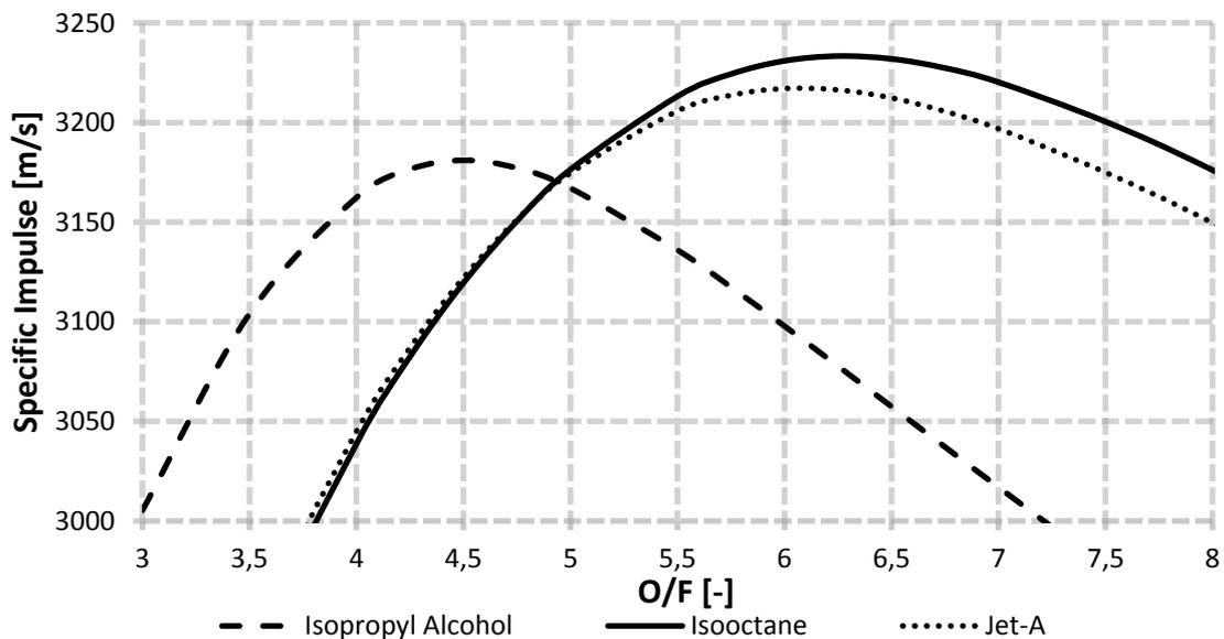
Figure 4. Theoretical specific impulse of fuels with 98%+ HTP,  $p_c=10$ bar,  $\epsilon=330$ .
