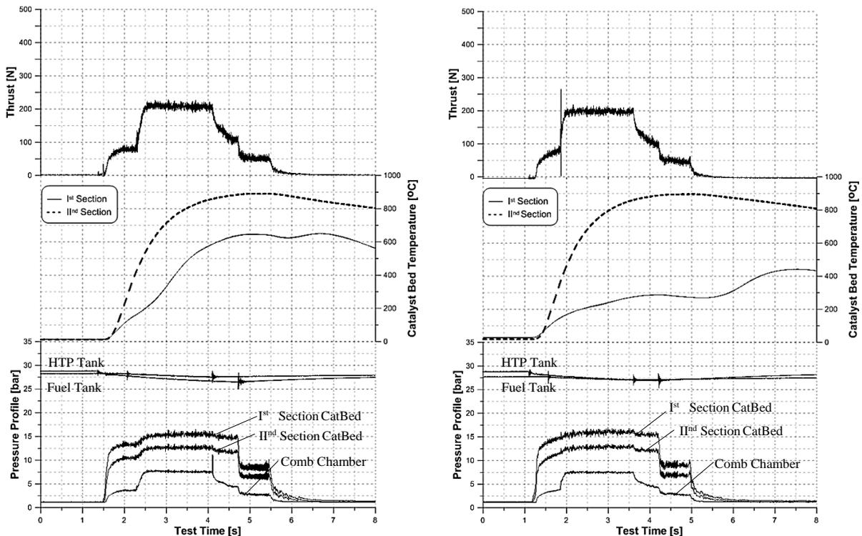
Figure 9. Measured parameters during the test of the kerosene ignition (4 injectors configuration).
