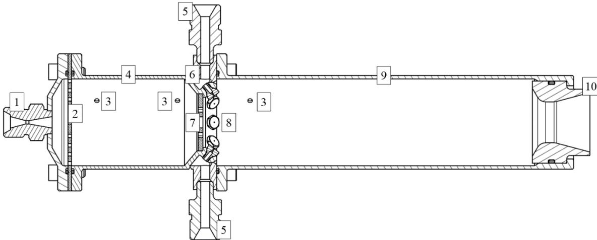
Figure 1. Engine cross section: 1-cavitating venturi, 2-HTP distributor, 3-measurement ports, 4-catalytic chamber, 5-fuel ports, 6-fuel collector, 7-HTP injector plate, 8-fuel injectors, 9-combustion chamber, 10-nozzle
