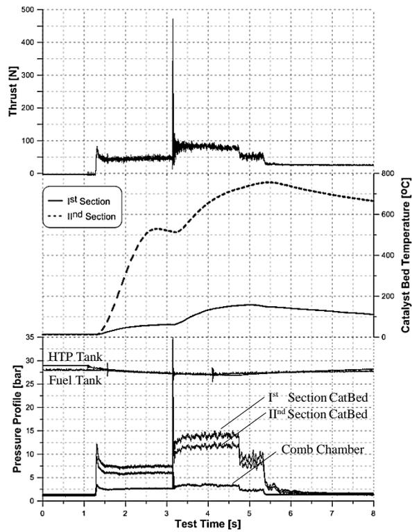
Figure 10. Measured parameters during the test of the isooctane ignition (8 injectors configuration).
