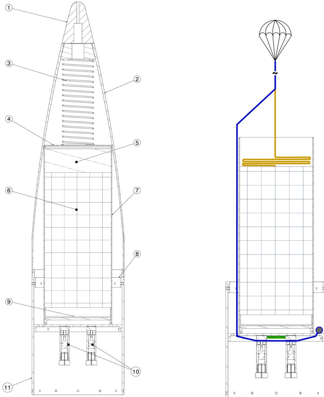
Figure 3: Complete scheme of the system before deployment (left) and with deployed drag parachute (right). 1 – top of the nose cone, 2- heat shield, 3 – spring, 4 – canister cover, 5 – drag parachute with pilot chute , 6 – main parachute, 7 – canister, 8 – pirotechnic separation ring, 9 – piston, 10 – riser cutters, 11 – rocket body. Blue line – drag parachute riser, orange – main parachute bridle to drag chute, green – main parachute riser.
