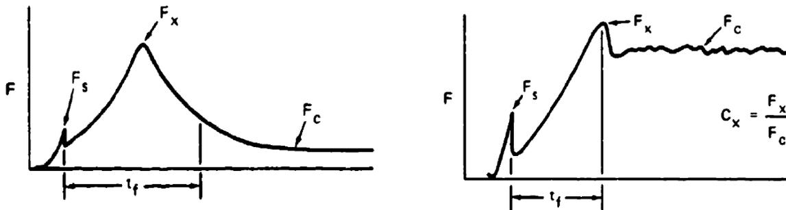
Figure 6: Differences between finite mass opening (left) and infinite mass opening [2].
