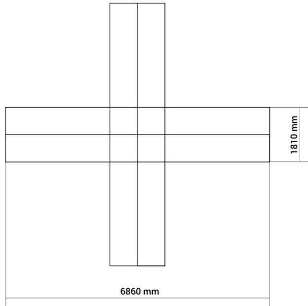
Figure 2: Constructed shape of main parachute.
