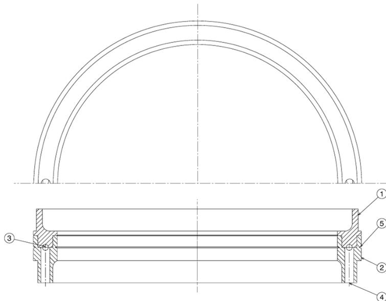
Figure 5: Pyrotechnic separation ring. 1 – top part, 2 – bottom part, 3 – PETN, 4 – mounting of detonating cap, 5 – weakening notch.
