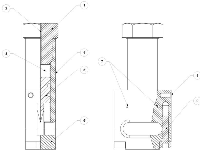
Figure 4: Scheme of designed riser cutter. 1 – plug, 2 – igniter channel, 3 – chamber, 4 – body, 5 – cutting knife, 6 – base, 7 – braking pins, 8 – mounting hole, 9 - connecting bolt.
