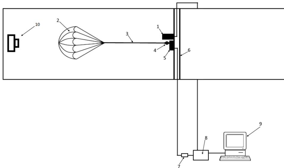
Figure 7: Scheme of test stand. 1 – parachute container, 2 – parachute canopy, 3 – riser, 4 – swivel, 5 – load cell, 6 – mounting bar, 7 – amplifier, 8 – measuring card, 9 – computer, 10 – camera.
