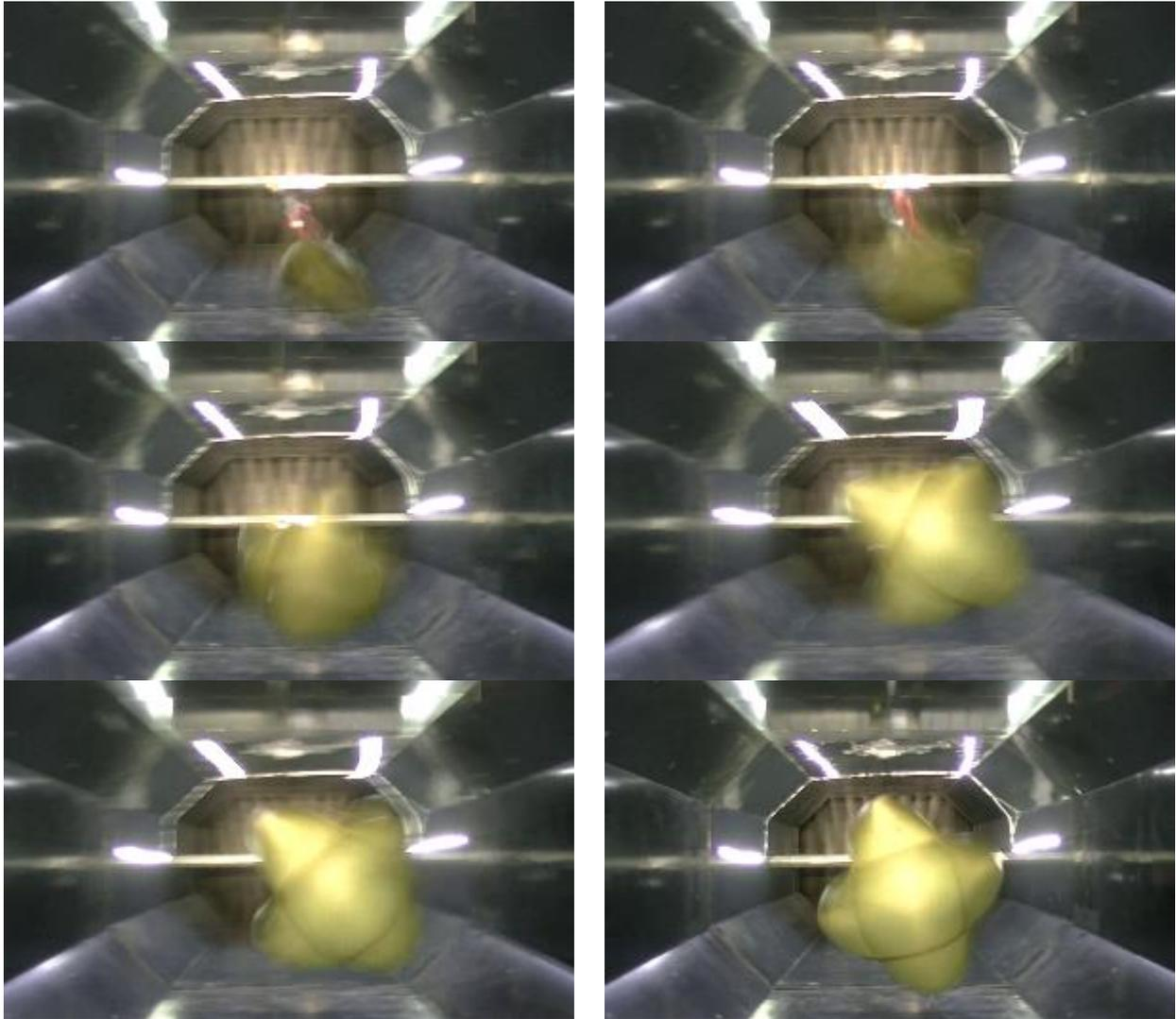
Figure 10: Inflation proces of cross parachute obtained from wind tunnel. Time interval – 0.02 s.
