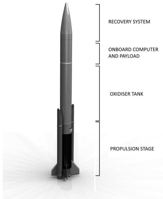
Figure 1: Render of the rocket model and sections.
