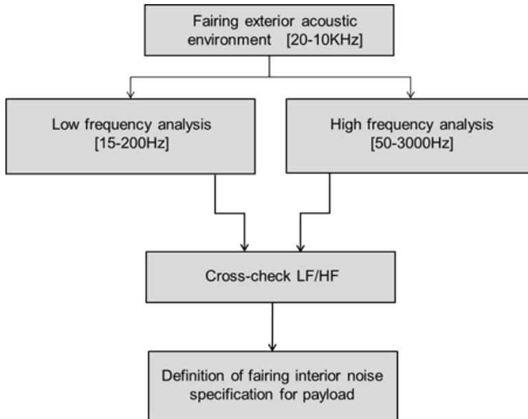
Figure 1. Vibroacoustic logic for payload interior noise specification
