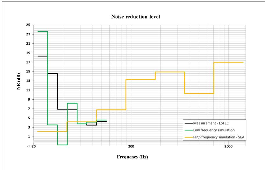
Figure 6. Comparison between simulation and ground test
