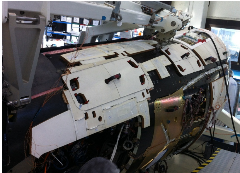
Figure 18: Jettison and lateral assembly integrated in Italy
