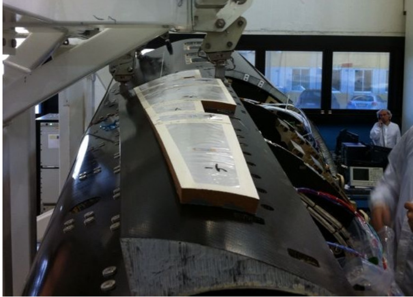
Figure 17: first integrated tiles of IXV ablative TPS.
