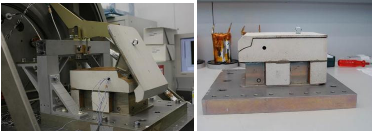
Figure 16: Umbilical connectors cover before and after qualification testing campaign.
