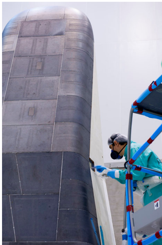
Figure 20: Last IXV ablative TPS tile being installed
