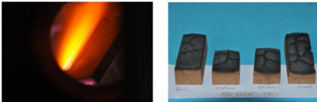
Figure 13: Flat plate test – 180Kw/m2
