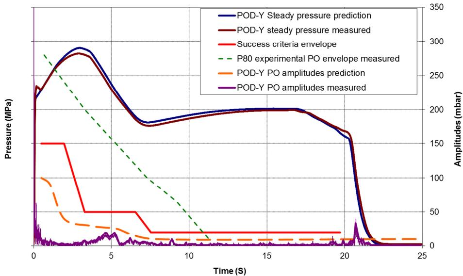
Figure 10: Unsteady pressure results – Comparison between prediction & results of POD-Y Bench firing test
