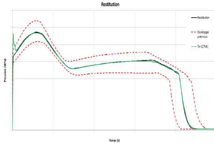
Figure 9: Pressure curve – Comparison between prediction & results of POD-Y Bench firing test
