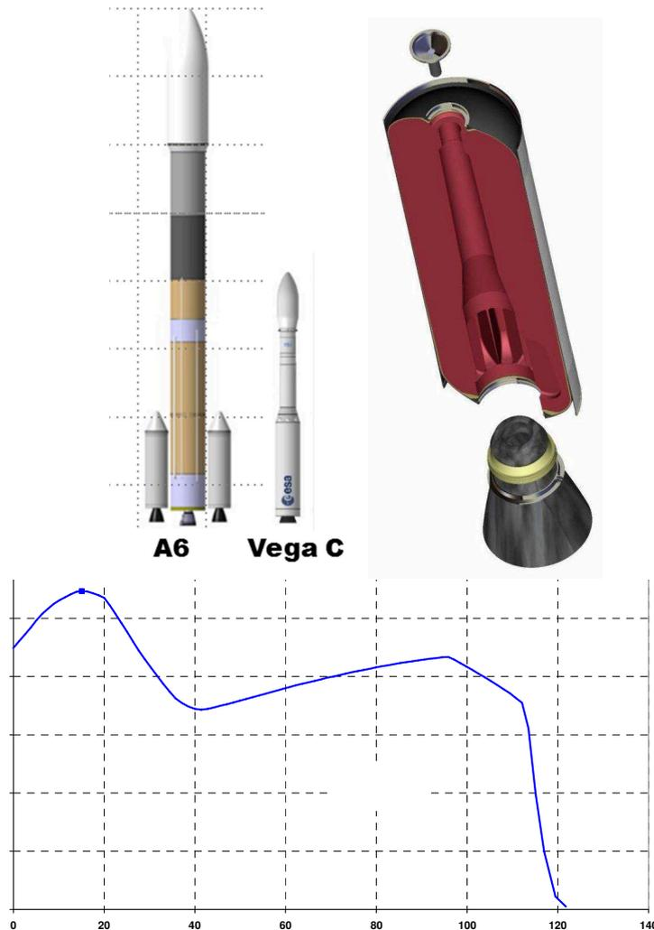
Figure 2 : Prototype SRM A6's global geometry and pressure evolution with time
