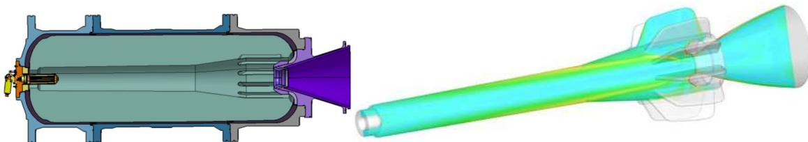
Figure 3: SRM A6's grain design and Stable flow (no vortices) obtained by computation
