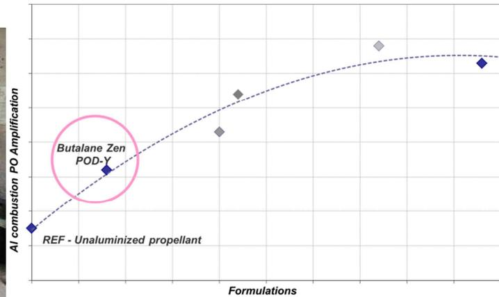
Figure 6: Results of Velocity Coupled T Burner – Al combustion contribution measure to PO amplification
