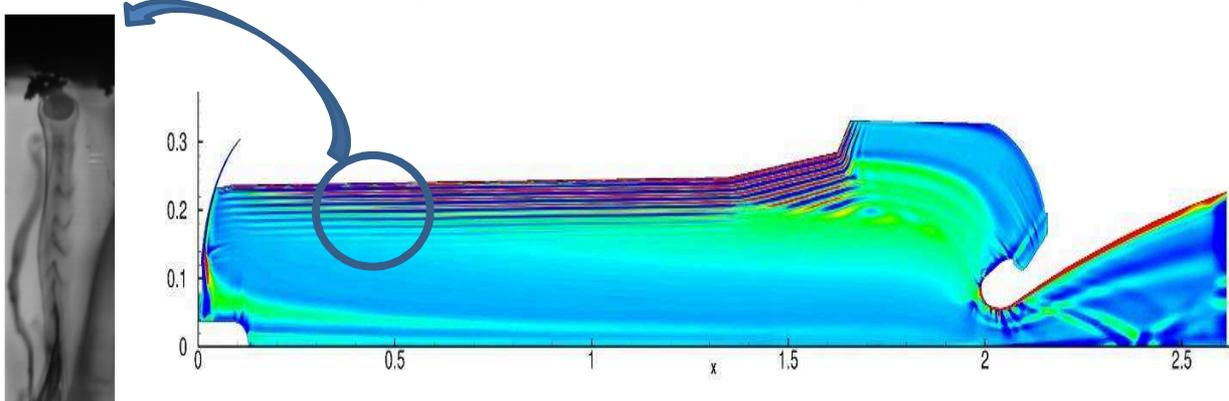
**Figure 5: Aluminium combustion close to propellant burning surface-** Experimental characterizations bench test bench and numerical effects modelled in the SRM combustion chamber (rotational field)
