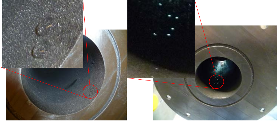
Figure 3: porosity test with water at 230 bar (left) and with Helium at 10 bar (right)
