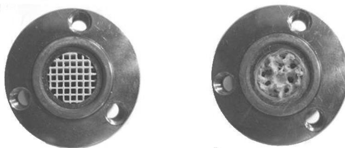
Figure 2: Photo of nude monolith and foam placed in the reactor
