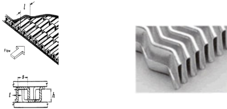
Figure 8 – View of off-set strip and wavy fins and their geometry
