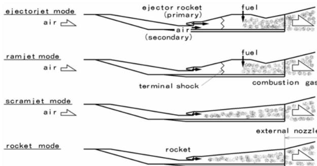
Figure 5: Conceptual Diagram of the RBCC engine
