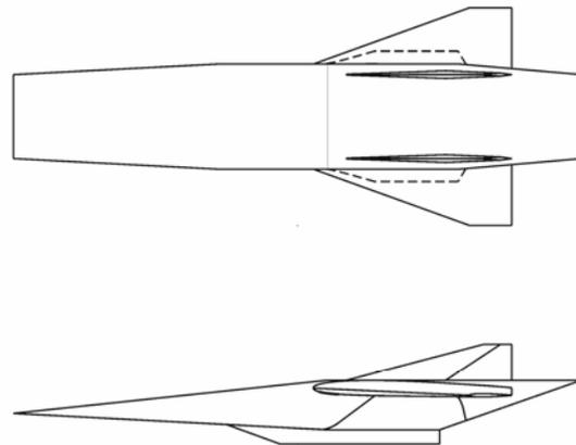
Figure 4: RBCC Engine-Mounted Vehicle
