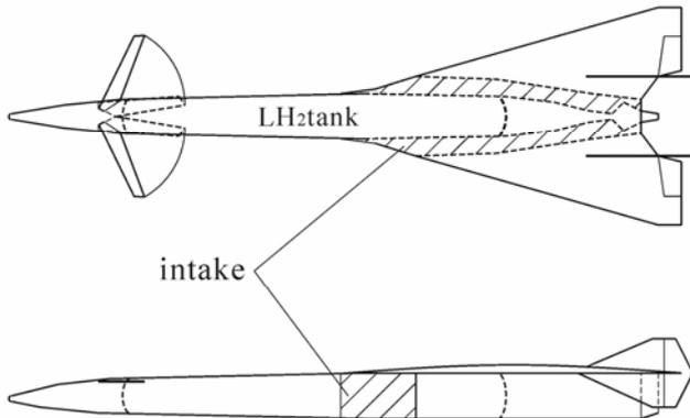
Figure 3: TBCC Engine-Mounted Vehicle
