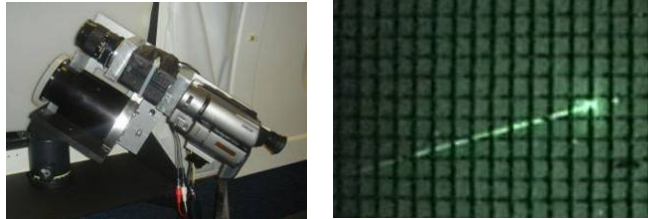
Figure 9: Camera and telescope (left) and tracking camera image of Stardust during entry (right).
