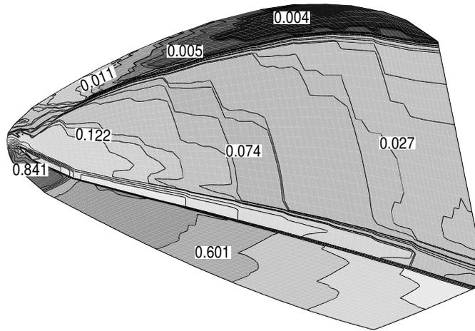
Figure 5: The pressure distribution ( $P/2q_\infty$ ) around body surface at  $M=10$ ,  $\alpha=35^\circ$ . Navier-Stocks equations
