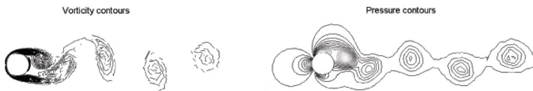
Figure 5: Flow lines for low Reynolds number
