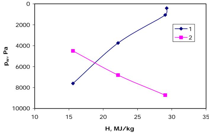
Figure 1: Pre-X re-entry trajectory (curve 1) and trajectory point for complete simulation of stagnation point heating. Curve 2 – Eq. (11)
