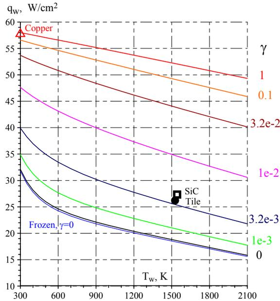
Figure 3: Heat flux envelope for the Pre-X test regime 2:  $Z_m=130$  mm,  $P_0=38$  hPa,  $N_{pl}=30.7$  kW. Measured heat fluxes to testing materials are shown by the symbols
