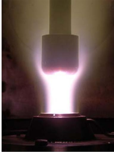
Figure 4: Stagnation point test configuration with precompression of subsonic high-enthalpy air flow at the plasmatron exit using water-cooled conical nozzle with 40-mm diameter throat
