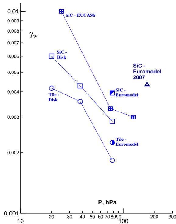
Figure 6:  $\gamma_w$  determined for SiC in different regimes using different TPM models. Tile-like model: SiC (squares,  $T_w = 1500 - 1600$  K); borocilicate coating (circles,  $T_w = 1470 - 1530$  K). Euromodel  $D_m=50$ mm: separate symbols, SiC (half-filled square,  $T_w = 1600$  K; triangle,  $T_w = 1650$  K); tile (half-filled circle,  $T_w = 1550$  K). Prior data for SiC<sup>11</sup> (crossed square,  $T_w = 1770$  K)
