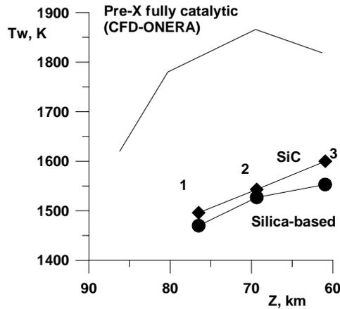
Figure 2: Stagnation point temperature of the Pre-X vehicle (fully catalytic surface), temperature of SiC and Silica-based surfaces under the IPG-4 plasmatron air test regimes 1 – 3
