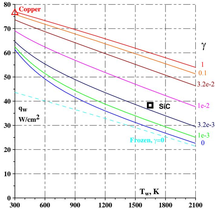
Figure 5: Heat flux envelope for the EXPERT test regime 1:  $Z_m=40$  mm,  $P_0=170$  hPa,  $N_{pl}=15$  kW,  $h_c=7.7$  MJ/kg,  $V_0=158$  m/s. Measured SiC surface temperature and rebuilt heat flux are shown by the symbol
