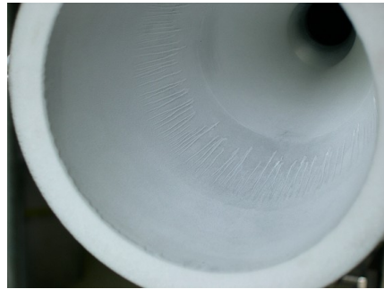
Figure 8 : frozen surface of the nozzle model
