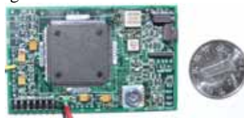
Figure 6: Integrated hardware of micro GNC avionics
