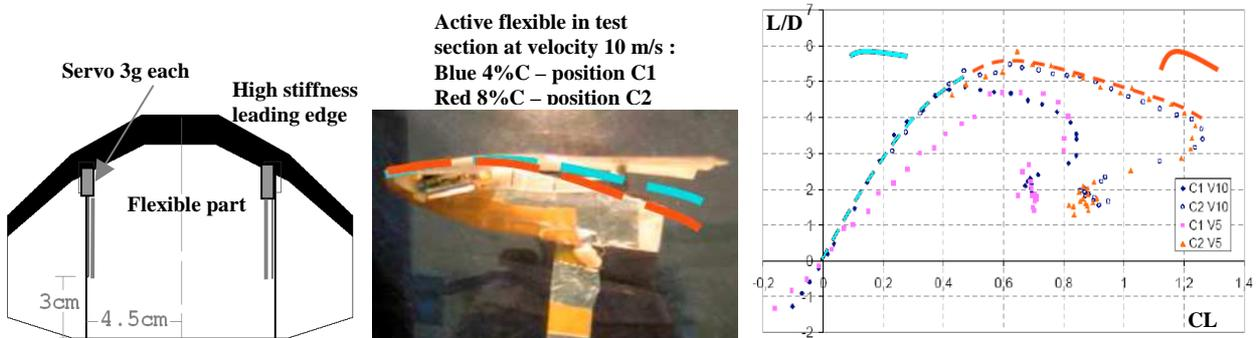
Figure 9: Active flexible wing controlled by servo-motors and L/D
