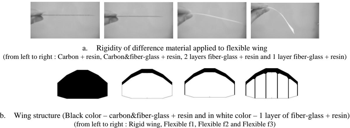
Figure 6: Rigidity of difference material applied to flexible wing
