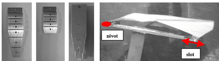
Figure 8: Fixation support (1<sup>st</sup>-type ‘A’, 2<sup>nd</sup>-type ‘B’ and 3<sup>rd</sup> and 4<sup>th</sup>-type ‘C’)
