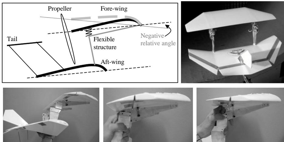
Figure 2: flexible biplane structure concept and Avilent model
