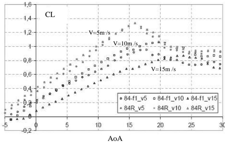
Figure 8: Effect of velocity on lift coefficient (V=5, 10 and 15m/s)
