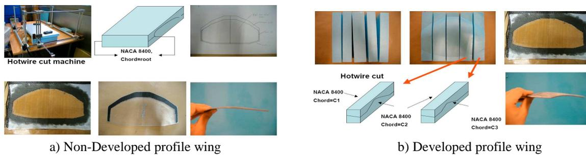
Figure 7: Fabrication process and Wing form
