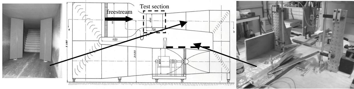
Figure 4: Longitudinal gust generator and low speed wind tunnel
