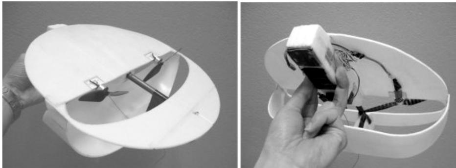
Figure 1: TYTO-30, low speed biplane pusher fixed-wing MAVs
