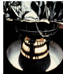
Figure 4: Novoltex ® carbon-carbon extendible nozzle extension (two translating cones) equipping a SRM.
