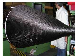
Figure 14: Advanced missile exit cone Naxeco ® preform: note the small entrance diameter and the large diameter ratio from top to bottom
