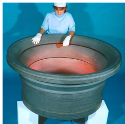
Figure 3: Novoltex ® carbon-carbon nozzle throat of Ariane 5 SRM
