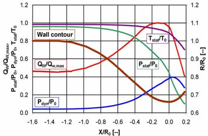
Figure 2: Axial distribution of typical thrust chamber parameters
