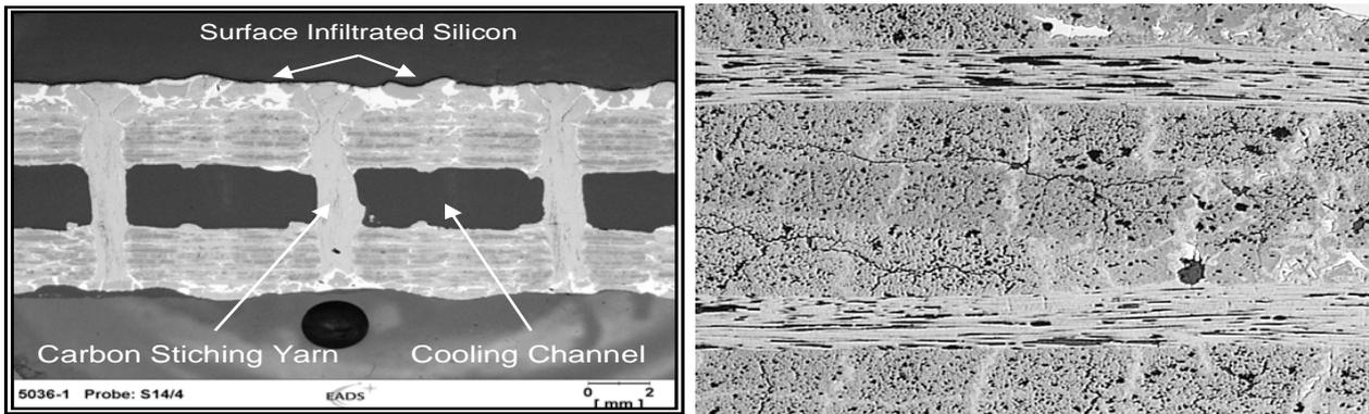
Figure 10: Sandwich structure with cooling channels (left) and cross-section of SICTEX<sup>®</sup> material (right)
