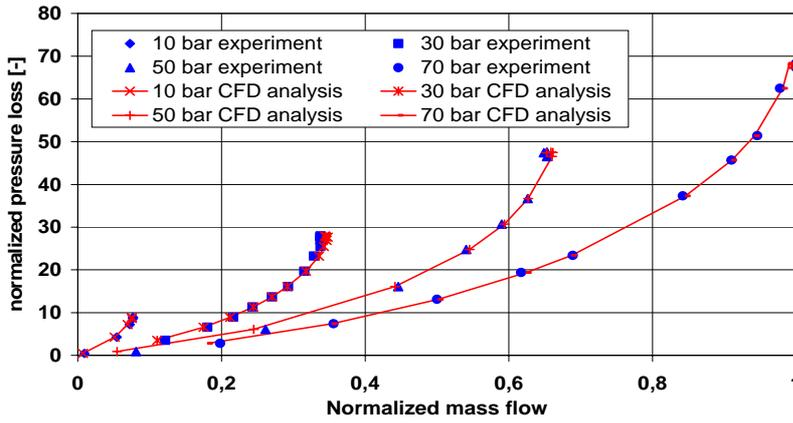
Figure 3: Comparison of experimental pressure results and CFD results with fitted Forchheimer parameters for cylindrical test sample for axial fluid flow parameters
