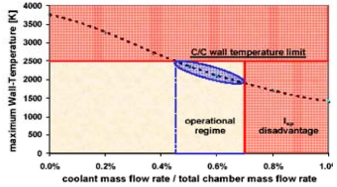
Figure 1: Operational domain of an effusion cooled TC liner
