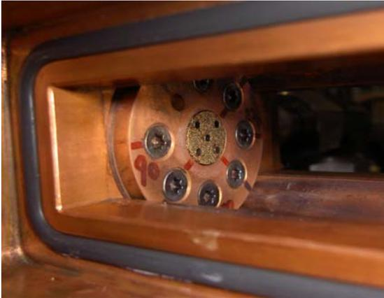
Figure 6: Porous penta-injector mounted in model combustor ‘C’
