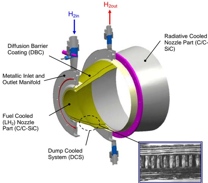
Figure 11: Fuel cooled CMC dual bell nozzle
