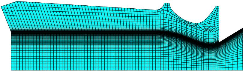
Figure 4: Meshing of the model in the area of the porous wall material
