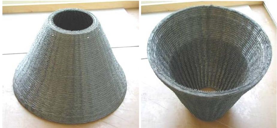
Figure 13: Braided and densified nozzle extension prototype
