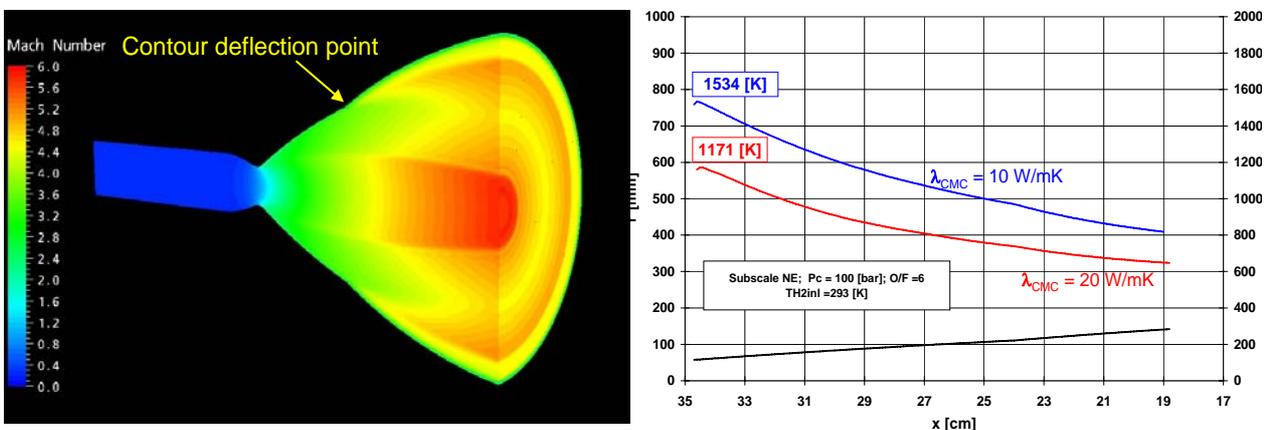
Figure 12: The thermal layout of the subscale FCCN has been conducted with Astrium's advanced heat transfer tools [15]
