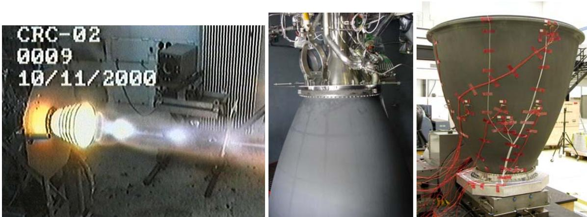
Figure 9: Hot test of nozzle extension (left picture), full-scale upper-stage nozzle extension on test facility (middle picture) and during vibration test (right picture)
