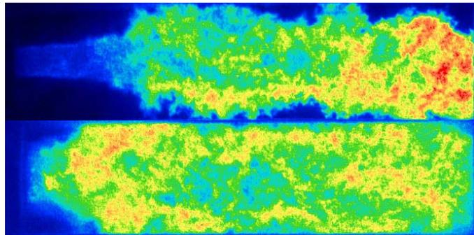
Figure 7: Comparison of the near face plate region of a shear coax (top) and porous (bottom) injector
