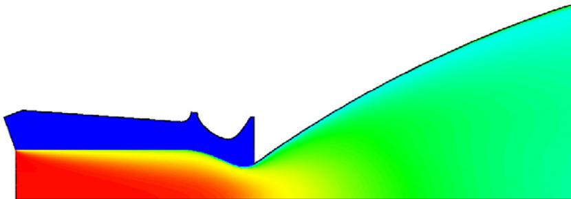
Figure 5: Temperature distribution along the liner wall
