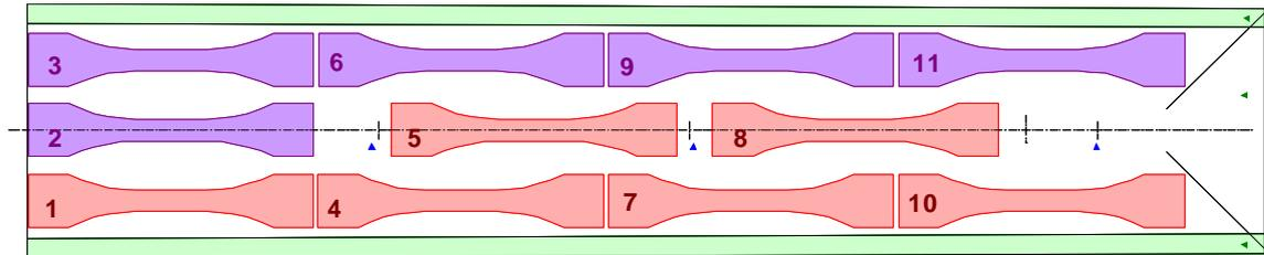
Figure 7: A500-CT1 and A410-CT1 cutting diagram
