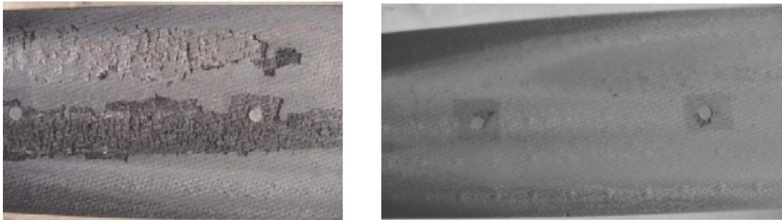
Figure 5: CERASEP® A410 seals, A410-CT1 showing seal-coat loss and A410-VT1 without any degradation
