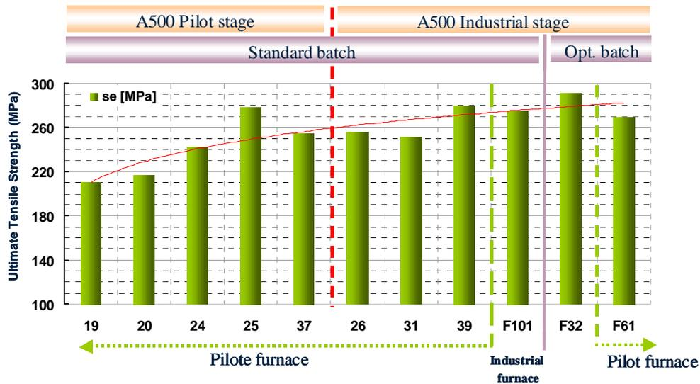
Figure 10: Plot of average tensile strength values measured on witness panels versus individual CVI furnace runs.
