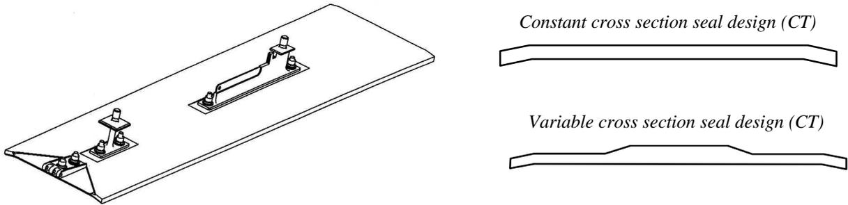
Figure 1: F100-PW-229 CMC seal schematics
