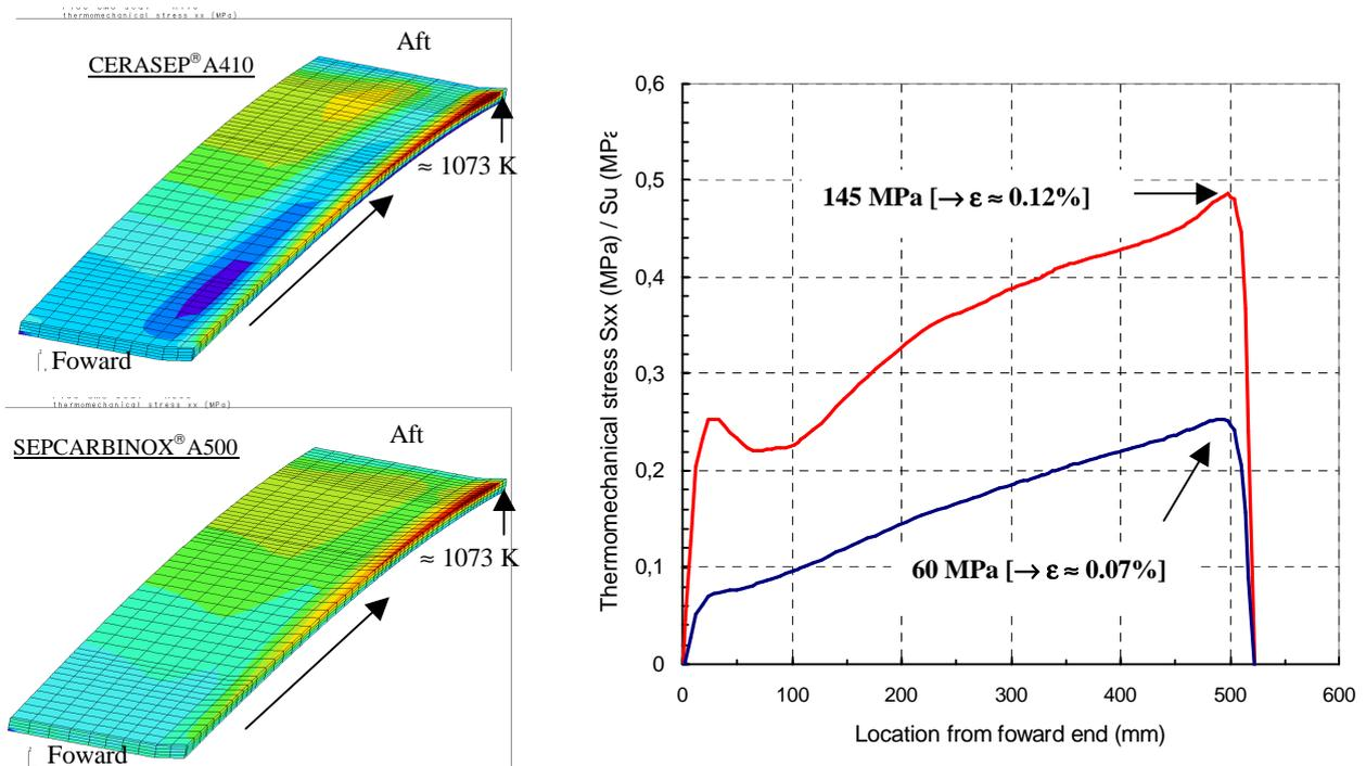
Figure 2: Calculated longitudinal stress
