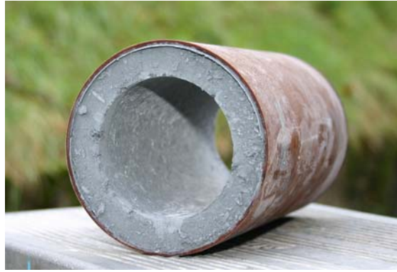
Figure 9 – BATES grain after storage
