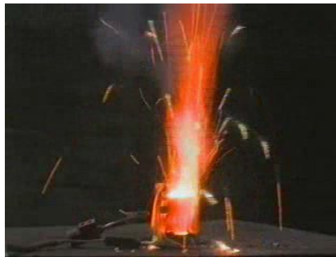
Figure 8 - Combustion of Mini-BATES grain at atmospheric pressure
