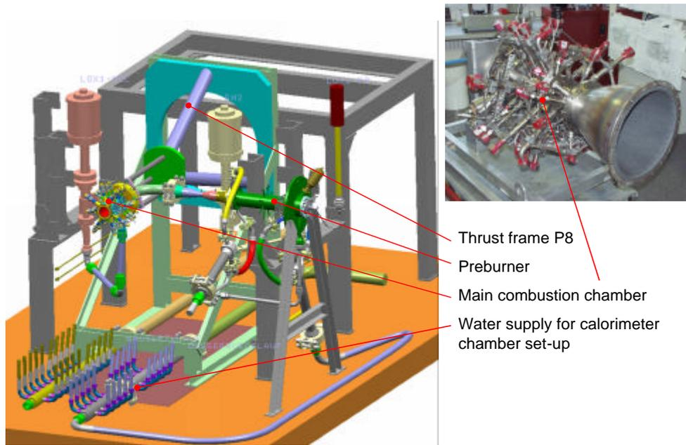
**Figure 6: Staged combustion pathfinder, with preburner and calorimeter main chamber set-up (top right).<sup>5</sup>**
