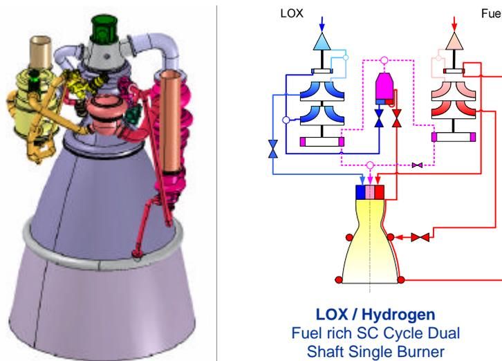
**Figure 1: LOX/H<sub>2</sub> reference engine architecture.**
