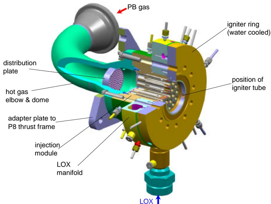
**Figure 8: Main combustion chamber injector head for 55 kN staged combustion demonstrator.**
