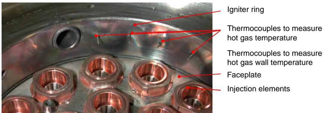
**Figure 7: Measurements foreseen for staged combustion injector faceplate.**
