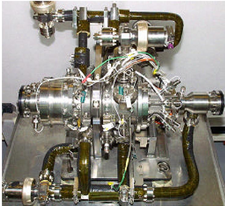
**Figure 5: TP Tech turbopump demonstrator.**
