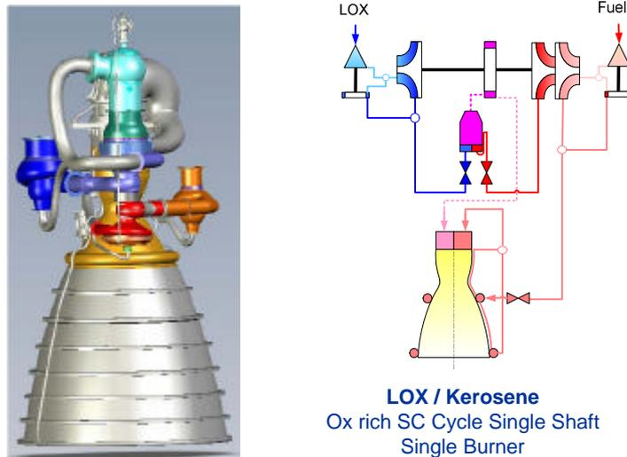
**Figure 2: LOX/Kerosene reference engine architecture.**
