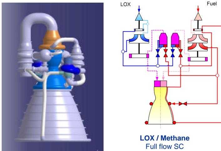
**Figure 3: LOX/Methane reference engine architecture.**
