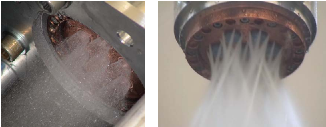
Figure 3. Preburner Cold Flow Tests: Kerosene-Side (left); Oxygen Faceplate Flow (right).
