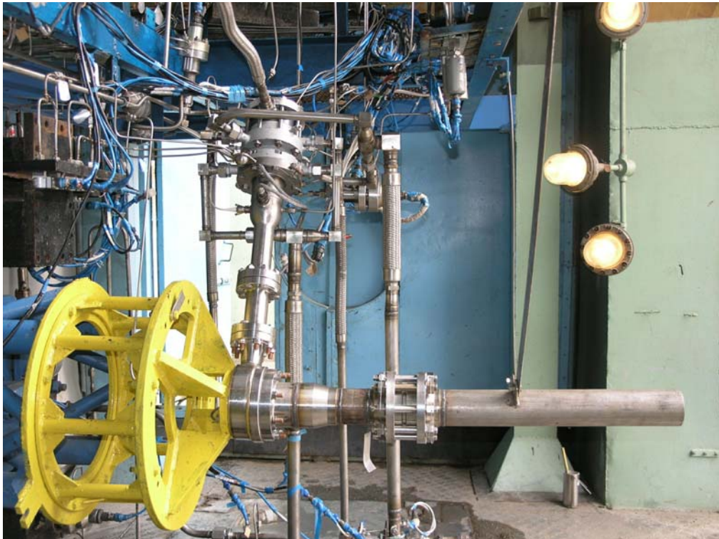
Figure 5. Preburner Installed on Test Bench with CC Simulator
