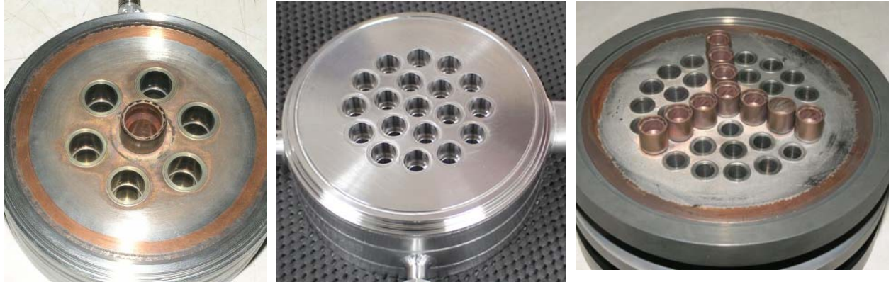
Figure 4. Subscale Main Chamber Injectors with 7 (left), 19 (center), and 37 (right) Elements
