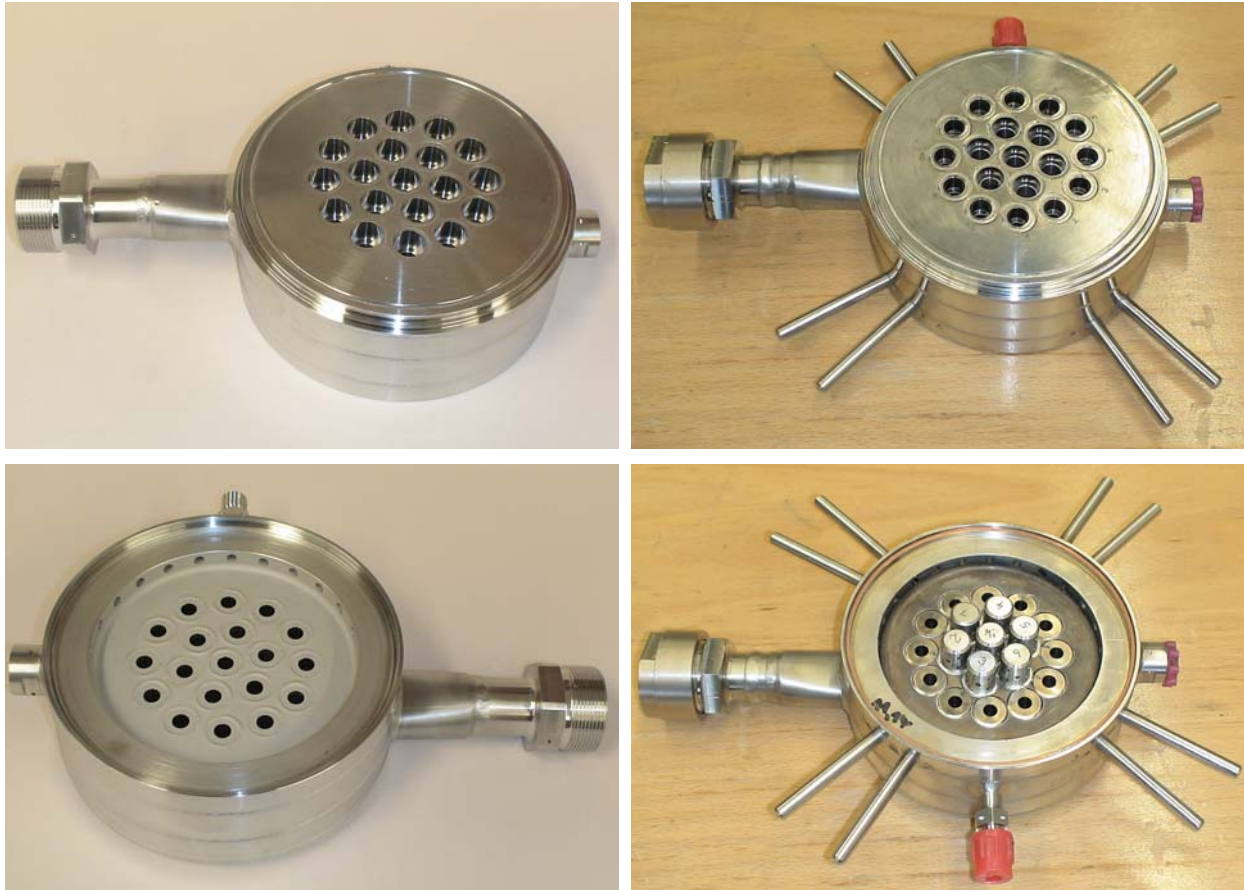
Figure 10. Main Injector in Initial (left) and Modified Configuration (right)
